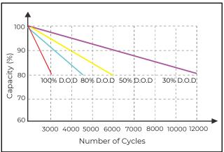
D.O.D. - depth of discharge S.O.C. - state of charge
